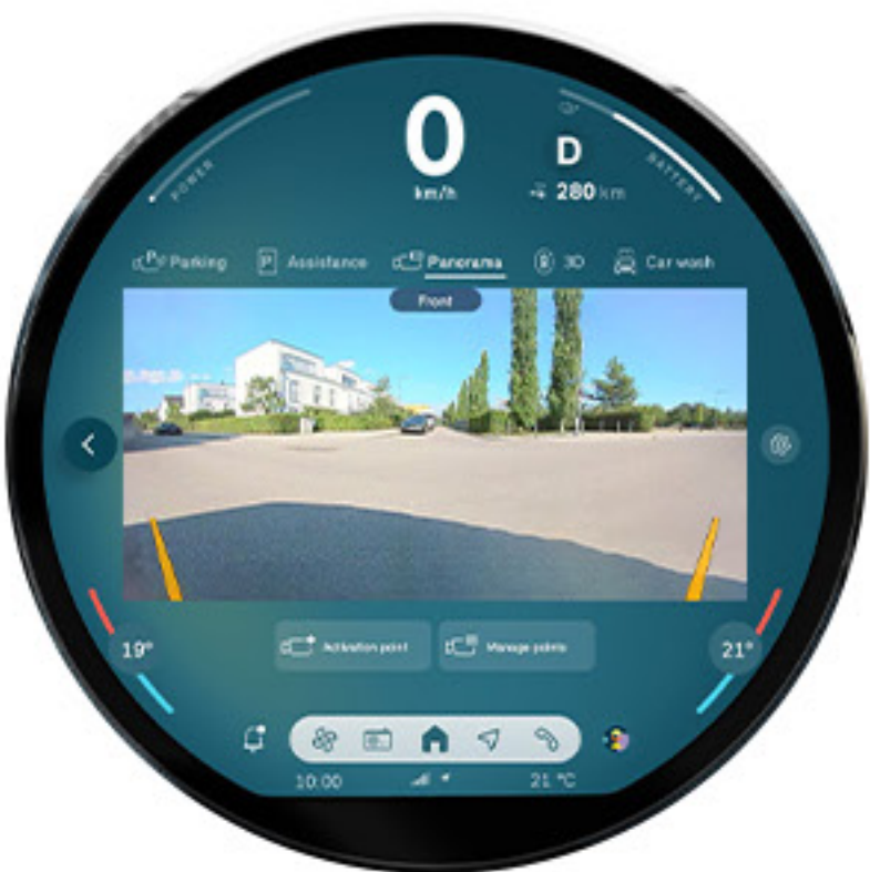
Parking Assistant Plus: Visual parking aid featuring Surround View cameras, Top View, Panoramic View and 3D View makes parallel and perpendicular parking on the road easier. The system completely takes over the steering, the accelerator, and the transmission. (Only for JCW Engines).
